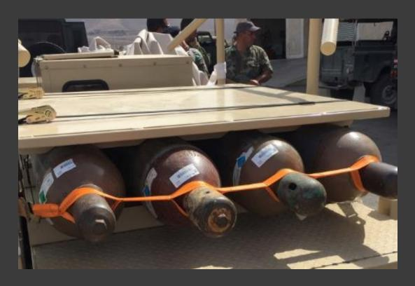
This particular design carries four full size helium bottles to fill the #18 Aerostat.
